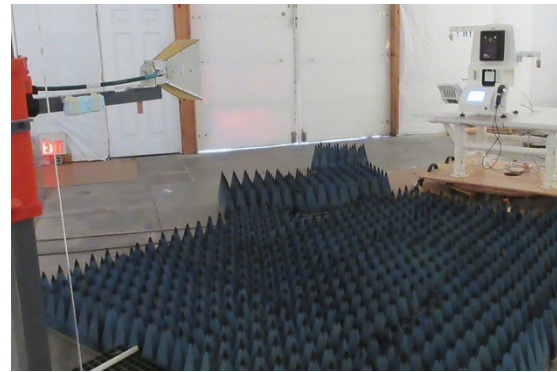
Testing for radiated emissions in host product at D.L.S. Electronic Systems, Wheeling, IL
