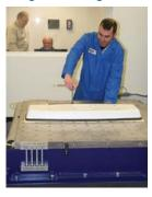
evaluating performance. D.L.S. also tests to SAE /Auto (vibration simultaneously with temp/ humidity), IEC and other vibration standards. For more information call Jack Black at 847-537-6400 or request a quote at
