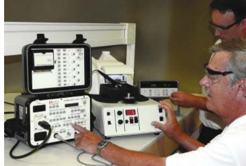
Performing Leakage Current Test on laboratory device
